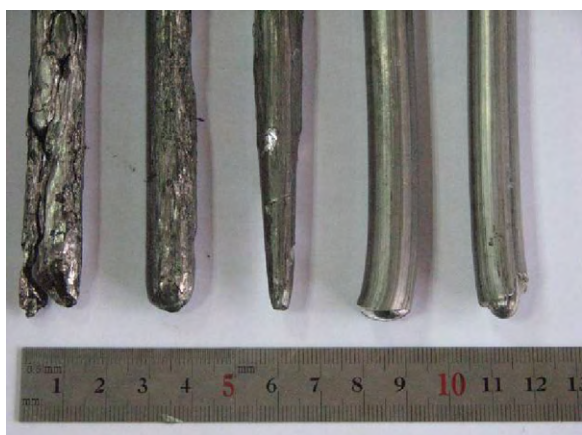
Fig. 2. The recycled specimens extruded from machined chips at 200 °C, 300 °C, 400 °C, 450 °C and 500 °C in sequence.
